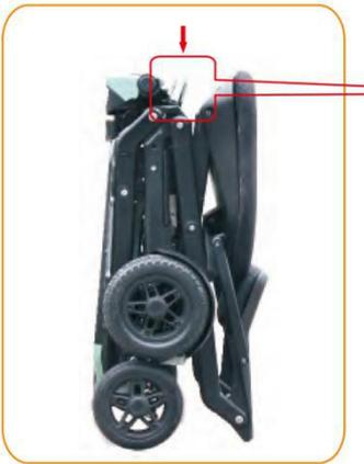
Push down the carry handle as far as possible and the scooter will start to unfold.
